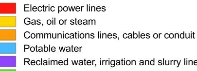
Reclaimed water, irrigation and slurry lines Sewers and drain lines
