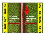
Respecting the tolerance zone protects buried utility lines from damage and also protects you from injury.
